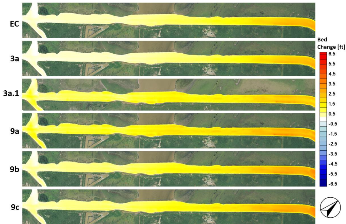
Figure 87. Sedimentation pattern in the West GIWW for all alternatives.
