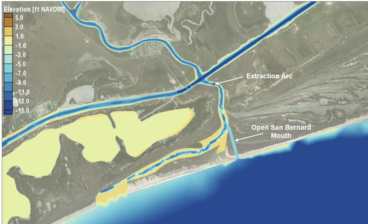
Figure 98. Extraction Arc Used for Inlet Stability Analysis
