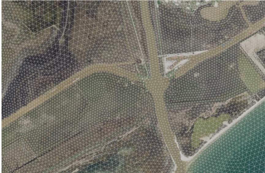
Figure 48: Resolution of Mesh at Project Site (approximately 65 m or 213 ft)
