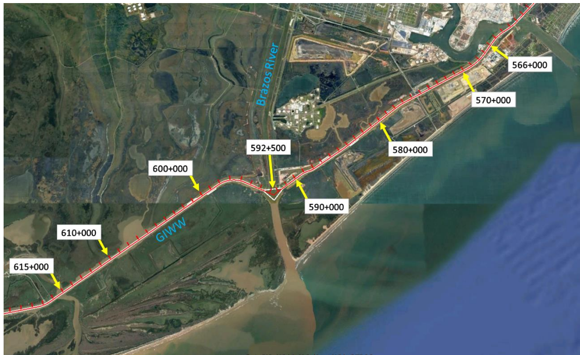
Figure 64. Station numbers along the GIWW channel alignment; survey and dredging data was investigated for the reach of channel extending from Station 566+000 to Station 615+000.
