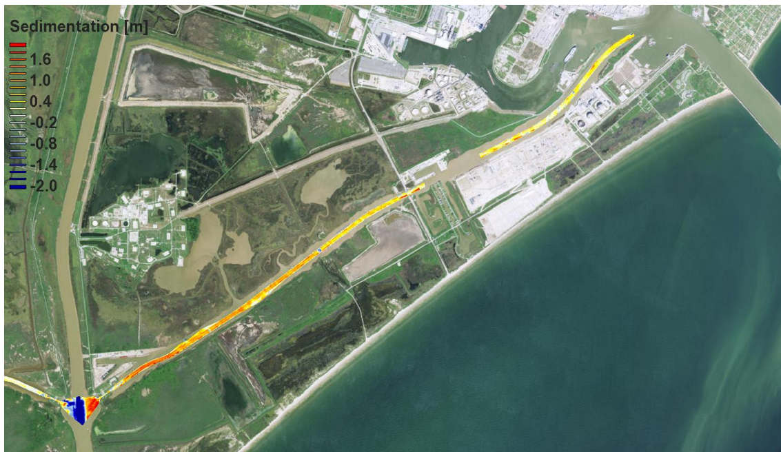
Figure 69. Sedimentation pattern in the E-GIWW due to Hurricane Harvey.
